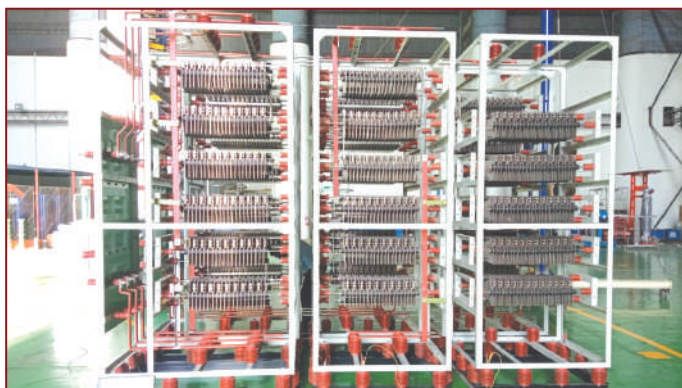
Resistor banks under Lightning Impulse Voltage Withstand Test
