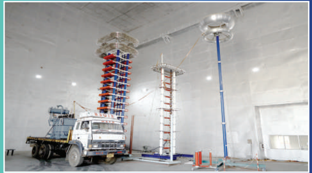
2400kV, 240kJ Impulse Voltage Generator
