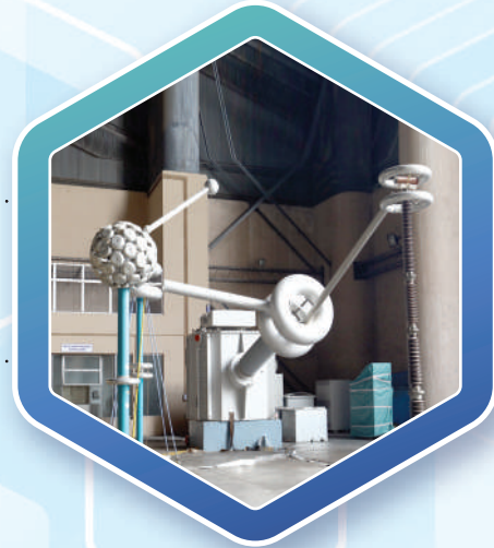
600 kV, 2000 kVA Transformer
