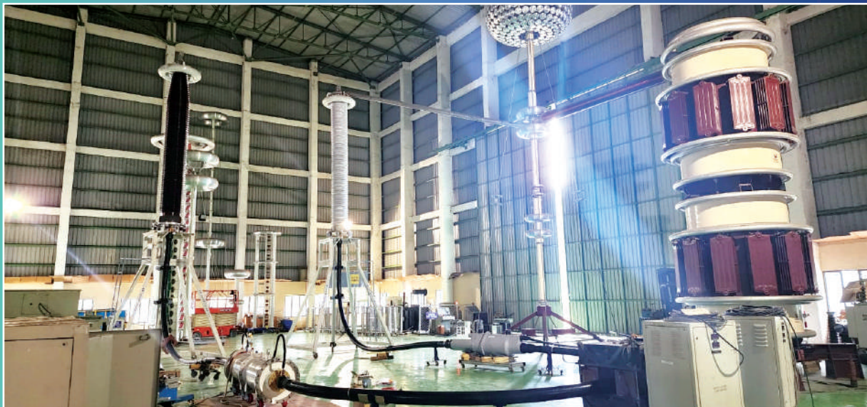
EHV Cable testing - 600 kV, 2400 kVA Series Resonant Test system
