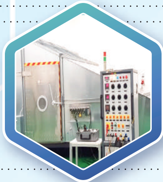
Test Set up for EMHF Immunity test by using GTEM
