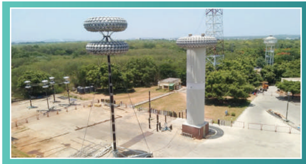
Aerial view of 5 MV, 5 kJ impulse voltage generator laboratory
