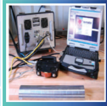
EMAT system for scanning of boiler tube wall thickness
