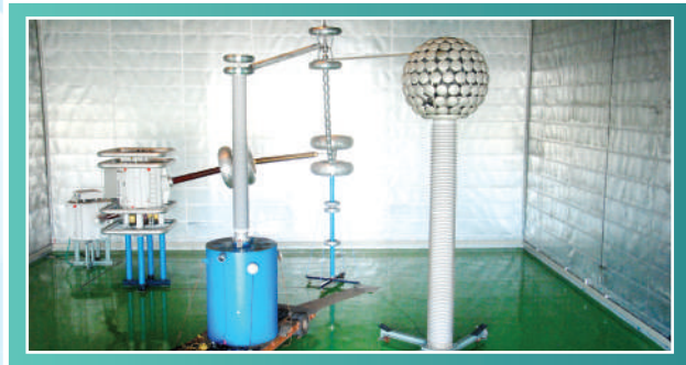
C and tan \delta test on 800 kV Bushing at UHV indoor double shielded laboratory
