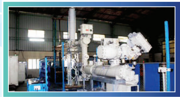
30V, 10000A Current Source for Accuracy Test on CT
