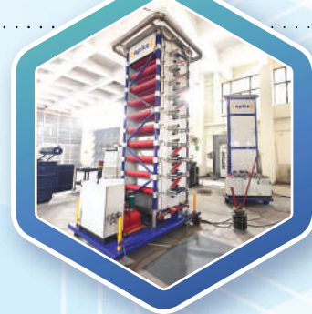
1000kV, 100kJ Impulse Voltage Generator
