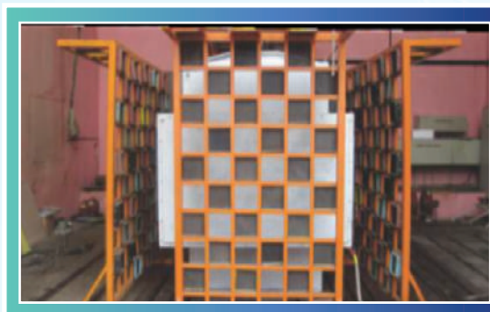
Internal Arc Fault Test on 33kV, 400A, Outdoor Kiosk Panel
